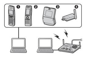
This feature allows you to access the Internet or another computer by connecting the units (①, ②, ③, and the base unit) with the USB cable or a USB adaptor (④) to your computer.
